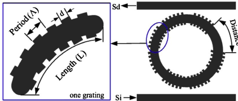
**Fig. 2.** Schematic of microring resonator with sidewall corrugation analogous to rectangular gratings.
